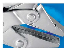
DO.888.300 Universal Parallel jaw pliers with side cutter, compound action Powerful pliers easily cuts outer bow of a facebow, serrated jaws assure non-slip grip while bending
